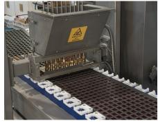
The presentation will cover the issues and solutions for accurate control of piece weights and addition of functional additives, for pectin and gelatin based gummies/jellies. The issues around the dosing of additives into syrups, in conjunction with depositor weight control setup will be examined and the technical solutions that are available to manufacture consistent infused products at capacities of 100lbs/hr. up to 2000lbs/hr.
